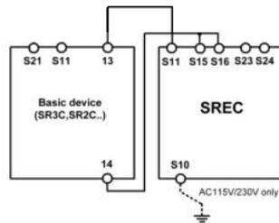
**Fig. 1: Connection of SREC to basic device**
