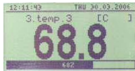
The current value of the measurement signal Height of the digits: 18 mm
