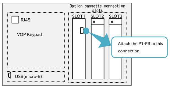
(3) Secure the P1-PB with the screw removed in (1)....
