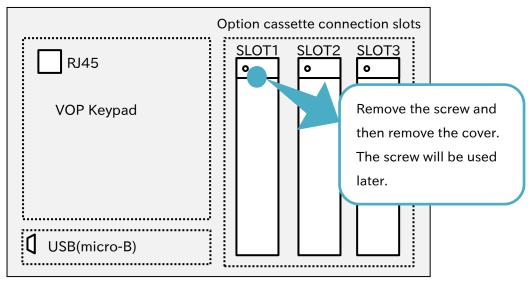
(2) Attach the P1-PB. The slots 2 and 3 have one more connection in the lower side. However, the P1-PB will not need that connection.
