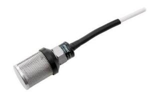
**Submersible level sensor CLS–23S** is developed as reliable and low-cost solution for limit level sensing of water (or water solutions) with miniature outer dimensions without the needs of any adjustment. It fully replaces the old type CLS–18S. The connection is done by means of two wires directly to a circuit with relay or to binary input of control system.
